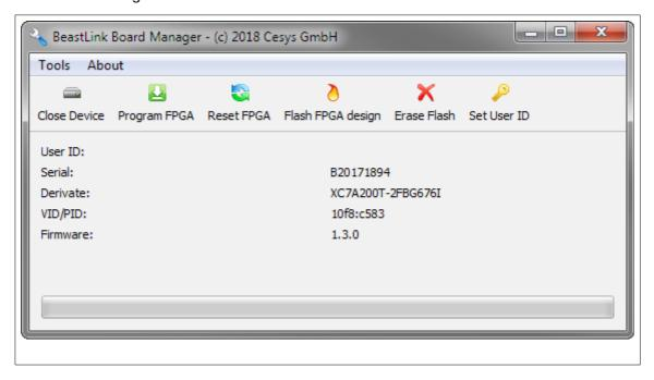
To work with a compatible board or module, use the mixed **Open Device/Close Device** button. If it shows the text **Close Device**, a device is currently opened. BeastLink Board Manager does **not** detect if the device is unplugged if it is opened.
