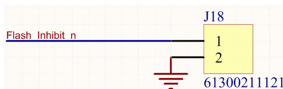
Figure 15: Jumper for Flash_Inhibit_n
